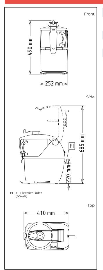
Electric Supply voltage: 200-240 V/1N ph/50/60 Hz Electrical power, max: 1.3 kW **Total Watts:** 1.3 kW Capacity: Performance (up to): 550 kg/Cycle **Capacity:** 5.5 litres Key Information: External dimensions, Width: 252 mm External dimensions, 485 mm Depth: External dimensions, Height: 505 mm **Shipping weight:** 30.5 kg
